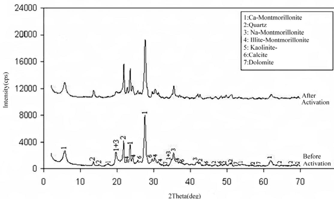
Fig. 2b: The Diffraction Patterns Of Kurşunlu Bentonite Before And After Activation.
