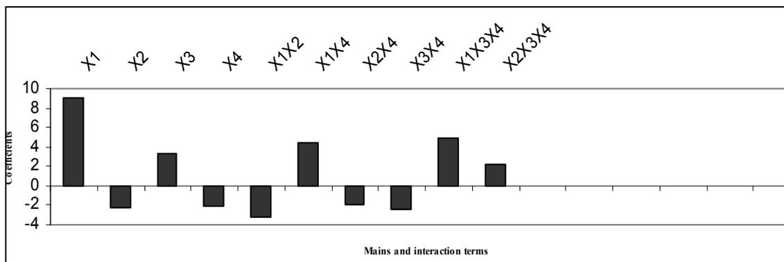
Fig. 1b: Significant Mains and Interaction Terms For Bleaching Capacity Of Kurşunlu Bentonite.
